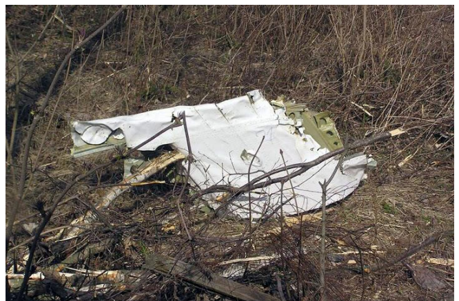
Fig. 17. A large size fragment of the airplane shell found on the Kutuzow Street roadside [15].
