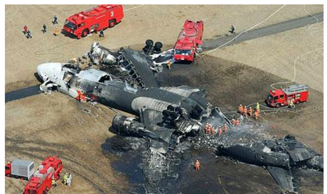
Fig. 9. The catastrophe of the MD-11 airplane in Tokyo, Japan on March 23, 2009. The airplane hit the ground, divided (perpendicularly to the airplane axis) into several segments. Then the plane exploded, the explosion occurred in the rear part, this part has been torn and opened longitudinally.
