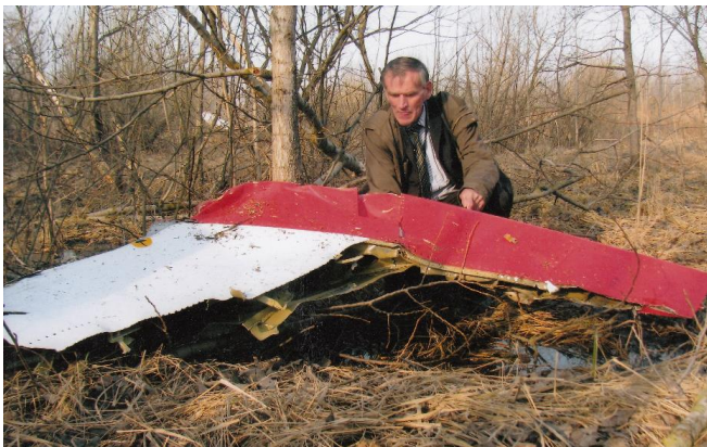
Fig. 18. A fragment of the left horizontal stabilizer lying in the woods about 5 meters from the Kutuzov Street. In the background, behind the trees, one can see the entire dart of the plane. Photo by Jan Gruszyński. Deformation of the detached parts excludes that detachment was due to a collision with a terrain obstacle.
