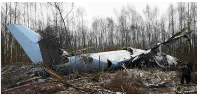
Fig. 6. The catastrophe of the Tu-204 airplane in Moscow on March 22, 2010. The catastrophe is of the 1A type -- the airplane hit the ground, no explosion.
