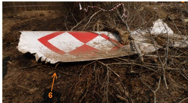
Fig. 25. The terminal part of the left wing (bottom shell) with the flap track fairings (6). In the background the right-hand-side horizontal stabilizer (3) [17]. The upper shell has been crushed and its pieces are in remote locations.
