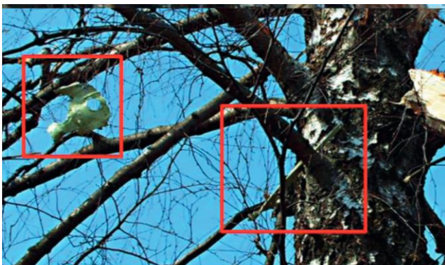
Fig. 30. Fragments of the left wing on the Bodin birch at the altitude of the breakthrough [10]. "Tin birds" have been detached from the aircraft, not less than several dozen meters earlier and much higher than the points they have been settled on.
