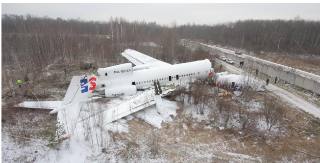
Fig. 5. The catastrophe of the Tu-154M airplane in Moscow on December 4, 2010. The catastrophe is of the 1A type -- the airplane hit the ground, no explosion.
