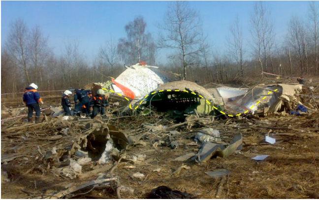
Fig. 3. The central part of the fuselage: from rung 40 till rung 64 [5]. The tear along the fuselage as well as the sides and the ceiling of the aircraft, that are flanged and thrown out, witness about a huge internal explosion. This kind of destruction cannot result from any external forces.
