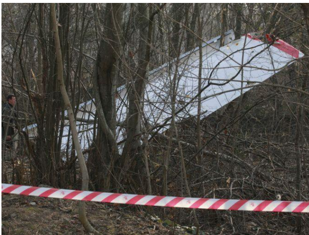
Fig. 29. The tip of the left wing lying in the location that is surrounded on all sides by the trees of height larger than 10 m [19].
