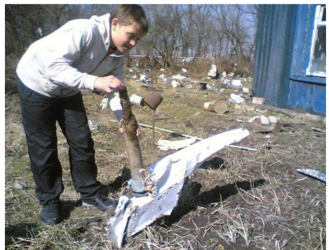
Fig. 13. The drive of the left wing outer flap with a part of the flap found at the foot of the Bodin birch [11].
