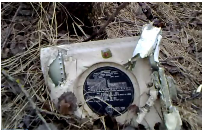
Fig. 19. A fragment of the main landing gear shock-absorber lying among the trees in zone 4 [16].
