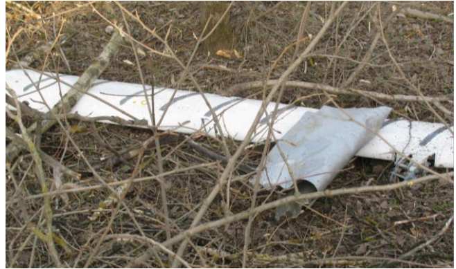
Fig. 20. The interceptor (deflector) of the left wing lying in the woods about 10 meters from the Kutuzov Street. On top a fragment of the slot is visible. Photo by Jan Gruszyński.
