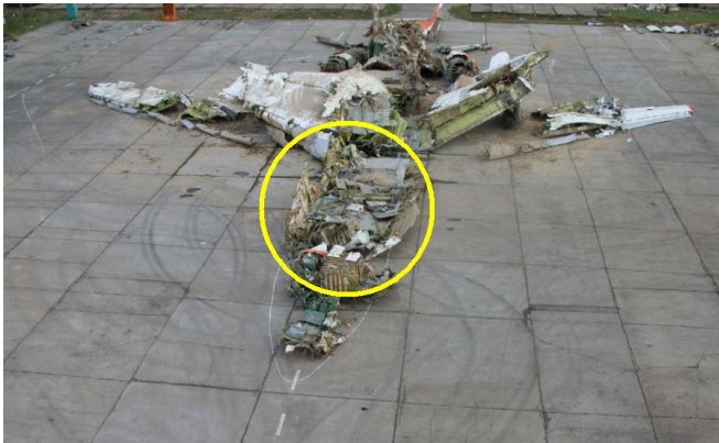
Fig. 4. The Tu-154M wreckage in the Smolensk airport [6]. It is evident, even after cutting off the ceiling as well as a large part of the sides, that the fuselage has been torn.
