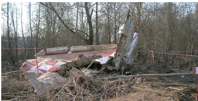
Fig. 23. The rest of the tail fin (vertical stabilizer) and the adjacent portions of the horizontal stabilizers [6]. The missing part of the horizontal stabilizers dropped off earlier.
