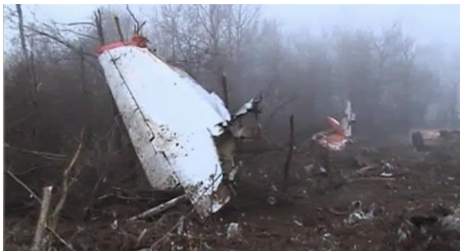
Fig. 22. The bottom surface of the terminal part of the right-hand-side horizontal stabilizer with the elevator. The leading edge is to the right. The lower part of the stabilizer lacks a fragment, that was detached in the direction of the flight [18].
