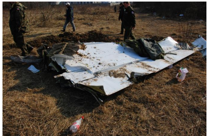
Fig. 21. Zone B5. The rear part of the left horizontal stabilizer (with the left elevator) [17].
