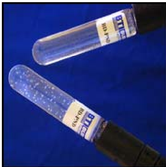
Figure 2.3-4. Photograph of bubble detectors that have (bottom) and have not (top) been exposed to neutrons.
