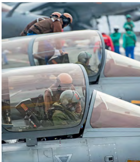
Above: Rafale M pilots strapping in prior to another mission. The Rafale's Mk16F ejection seat is reclined at 29°. Dassault Aviation/Katsuhiko Tokunaga
