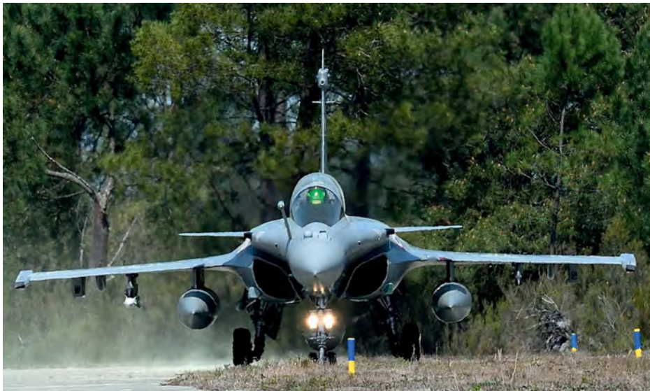
Above: With its AESA radar, Meteor and Mica missiles, powerful engines, remarkable agility and an advanced data-fusion system, the Standard F3R Rafale will prove to be a lethal foe in the air-to-air arena for years to come.
