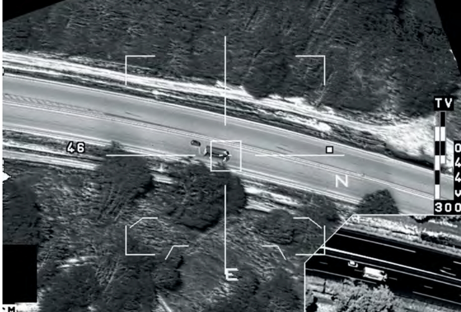
Above: The quality of the image provided by the TALIOS pod is said to be exceptional, much better than that of the Damocles, especially in daylight thanks to the adoption of a powerful TV sensor. Mounting the pod on the right forward-fuselage hardpoint ensures an excellent field of regard.
