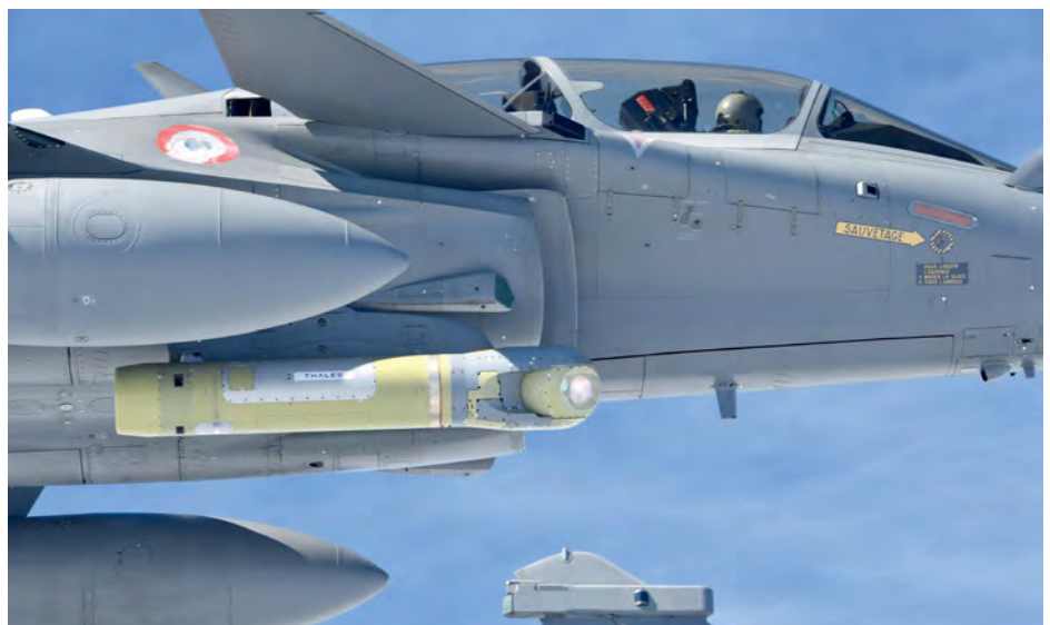
Above: A close-up of the new TALIOS targeting pod. The external shape of the TALIOS is similar to that of the older Damocles, helping cut integration costs thanks to a significant reduction in the number of sorties needed for flight envelope expansion.
