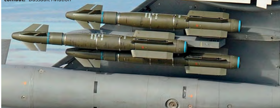
The Rafale can carry Hammer precision munitions on a triple launcher under each wing. Rafales are expending huge quantities of weapons in combat. Dassault Aviation
