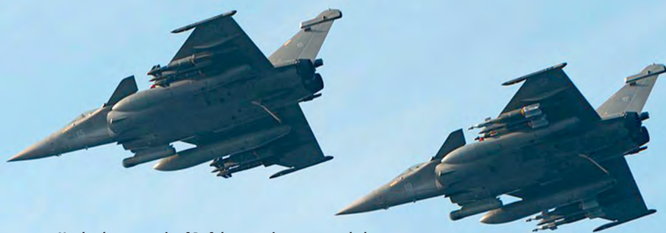
Hooks down, a pair of Rafales carrying unexpended ordnance enters the circuit at precisely 657ft (600ft above the deck, and another 57ft above the water). The leader is armed with four Hammers and the wingman, four GBU-12s. Marine Nationale
