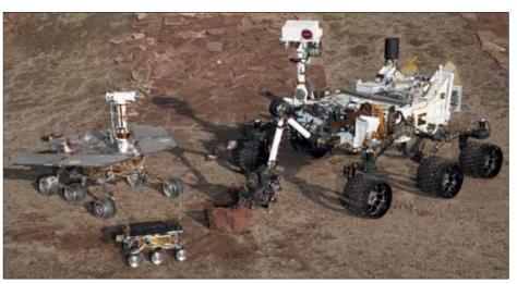
1: The increasing size of Mars rovers, from Pathfinder (front left), a Mars Exploration Rover (left), to Mars Science Laboratory (right). This increase in size (and cost), contrary to predictions that improved technology will result in smaller and cheaper robots, is mandated by the nature of the martian surface and complexity of exploration objectives. Human missions would be even larger and more expensive, but, crucially, much more capable. (NASA/JPL-Caltech)
