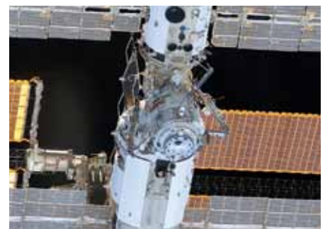
Pirs Module location at Service Module nadir.
