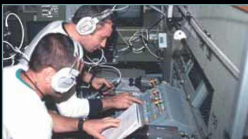
Crew uses Progress Remote Control workstation in SM.
