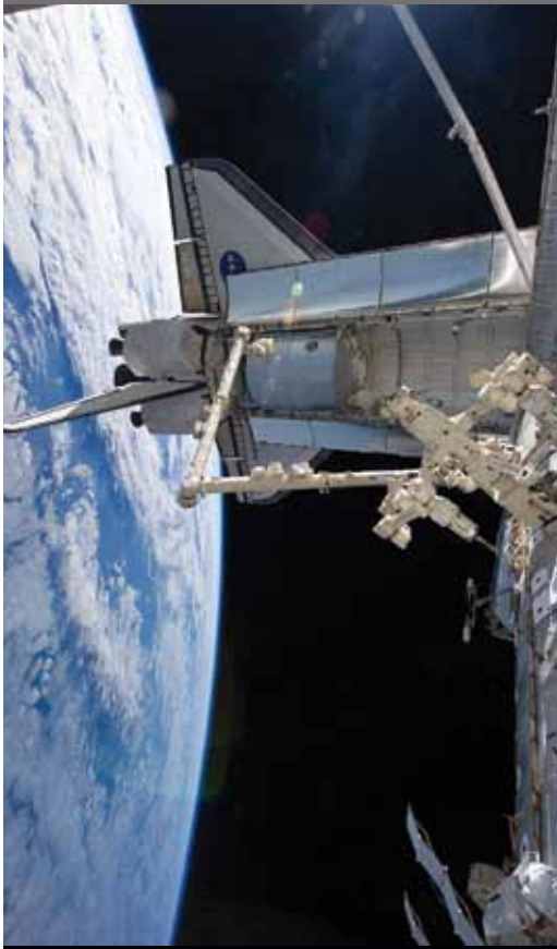
The station's robotic Canadarm2 grapples the Leonardo Multi-Purpose Logistics Module (MPLM) from the payload bay of the docked Space Shuttle Discovery (STS-131) for relocation to a port on the Harmony node of the ISS. Earth's horizon and the blackness of space provide the backdrop for the scene. Canadian-built Dexter, also known as the Special Purpose Dexterous Manipulator (SPDM), is visible at bottom center.
