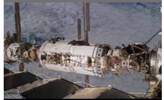
View of the FGB on orbit flanked by the Service Module and PMA-1.
