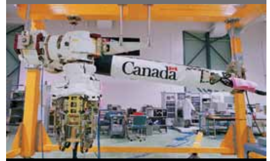
SSRMS during testing.
