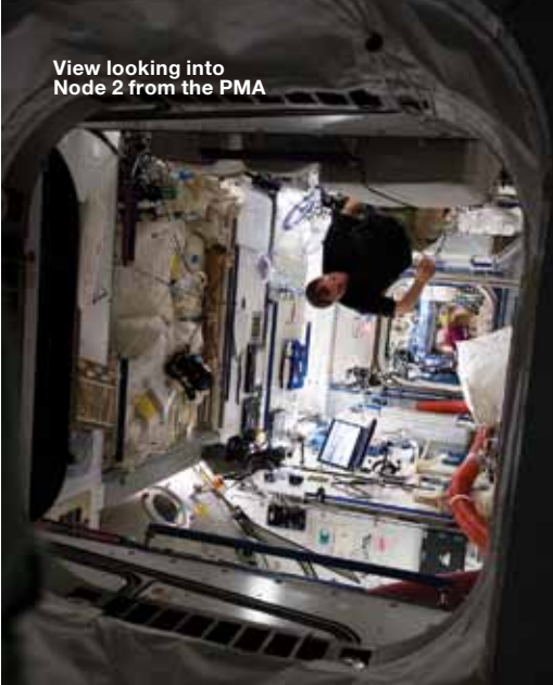
Permanent crew quarters were added to Node 2, permitting expansion of the total ISS crew size to 6. Crew quarters are rack-sized containers built as small state-rooms for the off-duty crewmember. Each crew quarter contains lighting, Station Support Computer (SSC) laptop connectivity, power, fans, ventilation, and caution and warning.
