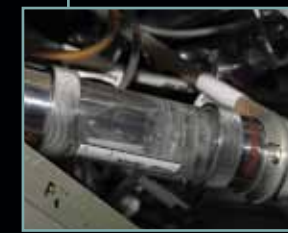
The Russian Condensate Water Processor is known as the SRV-K, equivalent to the US WPA, processes the condensate that is reclaimed by the SKV.
