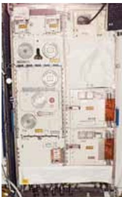
Used to perform space biology experiments on microorganisms, cells, tissue cultures, small plants, and small invertebrates.
