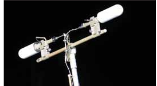
UHF antenna on the P1 Truss.
