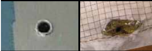
A 1.4-mm-diameter (inside) hole found in March 2001 in an ISS mini-pressurized logistics module outer bumper panel (no damage reported to pressure shell).
