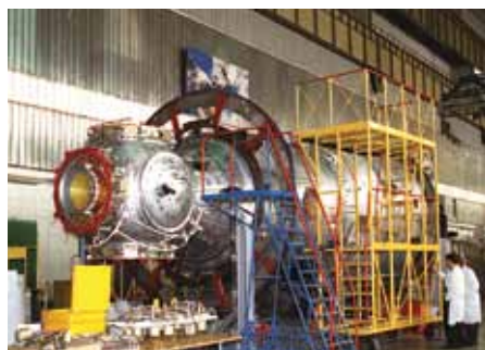
The SM's hull under construction at Khronichev State Research and Production Space Center in Moscow.
