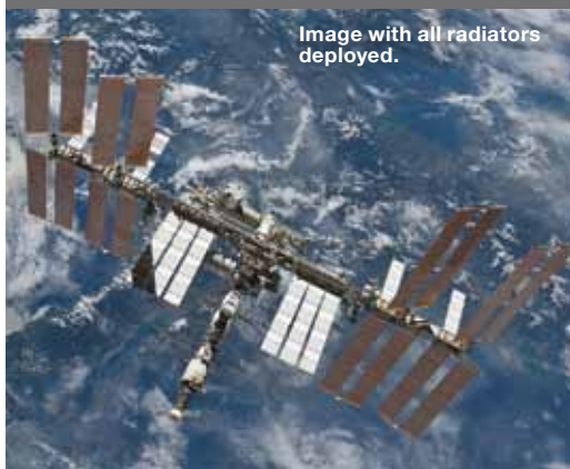
Starboard radiator panel after deployment.
