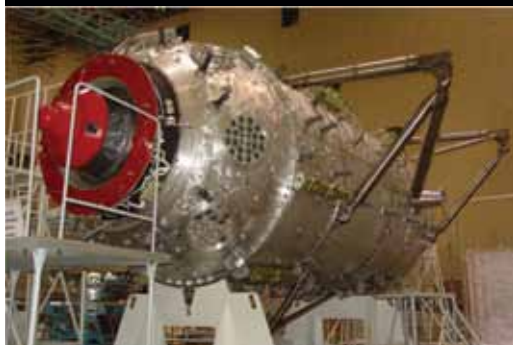
MRM1 Flight Article being assembled.
