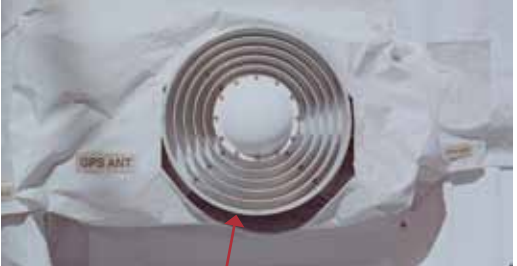
GPS antenna on S0 Truss.
