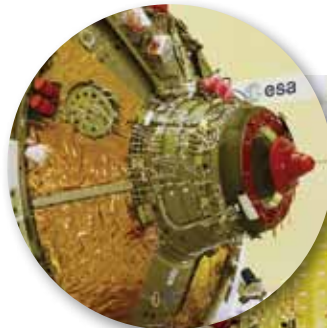
Russian-built probe and drogue docking system.
