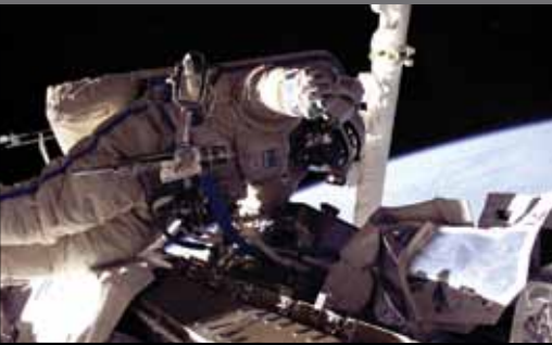
Crewmember Mike Fincke replaces the Remote Power Controller Module (RPCM) on the S0 Truss.
