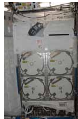
A refrigerator/freezer for biological and life science samples.
