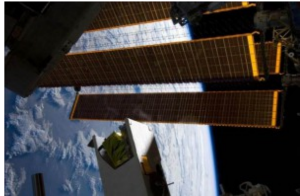
Data from the Hyperspectral Imager for Coastal Oceans (HICO)—pictured here as installed on the Japanese Experiment Module Exposed Facility—used in concert with field data can help researchers better understand and communicate coastal water quality. (NASA)
