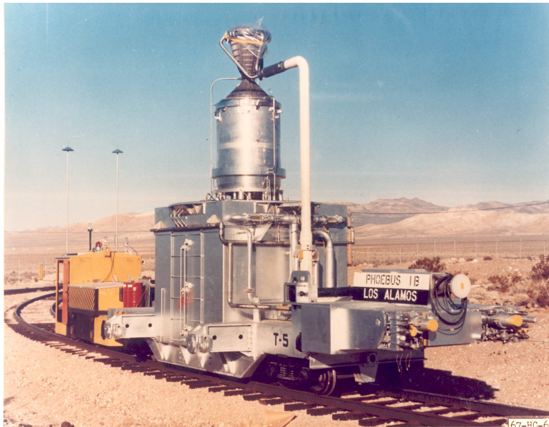
Phoebus-1B Engine Operated at Full Power and Thrust ( \sim 1500 \text{ MW}_{\text{th}} , 75 \text{ klb}_f , \sim 30 \text{ min} ) February 23, 1967
