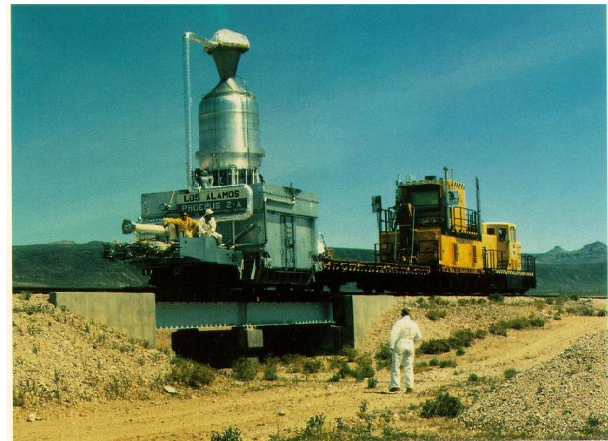
Phoebus-2A Engine Nominal Design Parameters \sim 5000 \text{ MW}_{\text{th}} , \sim 250 \text{ klb}_f , 820 \text{ sec } I_{\text{sp}} Four Tests in June - July 1968 Peak Power 4082 \text{ MW}_{\text{th}}
