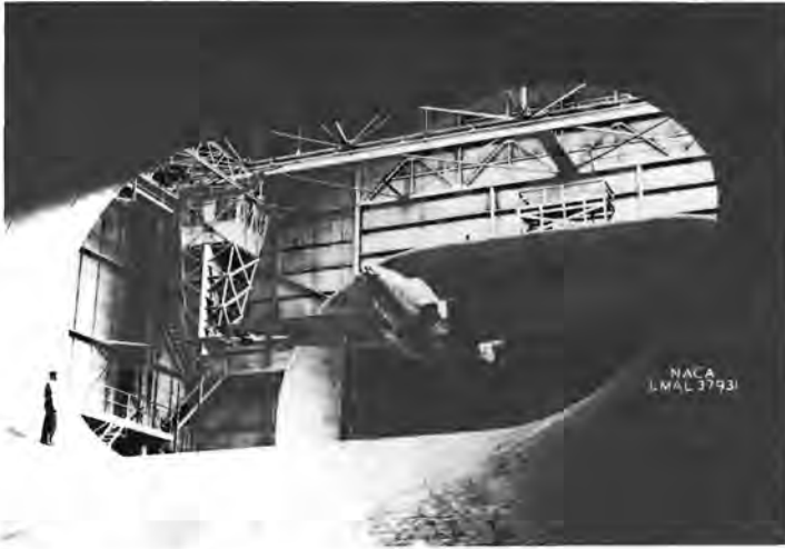
Drag cleanup of the Bell P-59, America's first jet airplane, in the Full-Scale Tunnel, May 1944.
