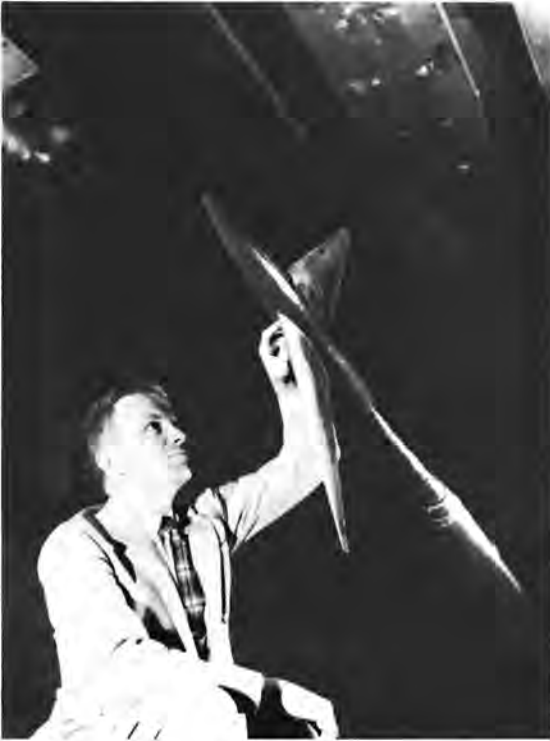
Richard T. Whitcomb examines a model based on his transonic area rule in the 8-Foot HST, April 1955.
