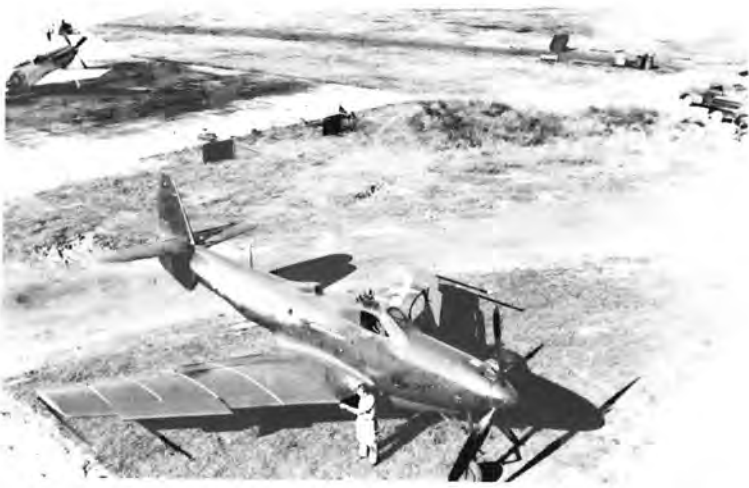
The L-39 was a purely experimental version of the Bell P-63 Kingcobra fighter designed to study the low-speed handling characteristics of swept wings, December 1946.
