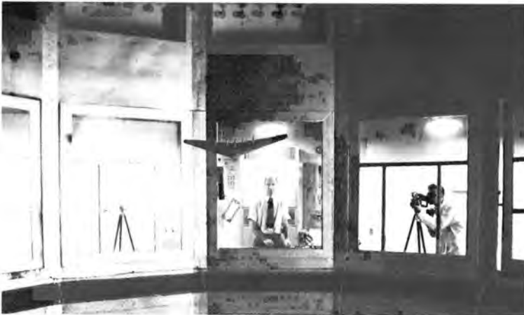
A model of the Northrop XB-35 flying wing was tested in the 20-Foot Spin Tunnel in 1943.
