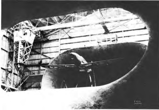
The P-51 Mustang is tested in the Full-Scale Tunnel, 1943.
