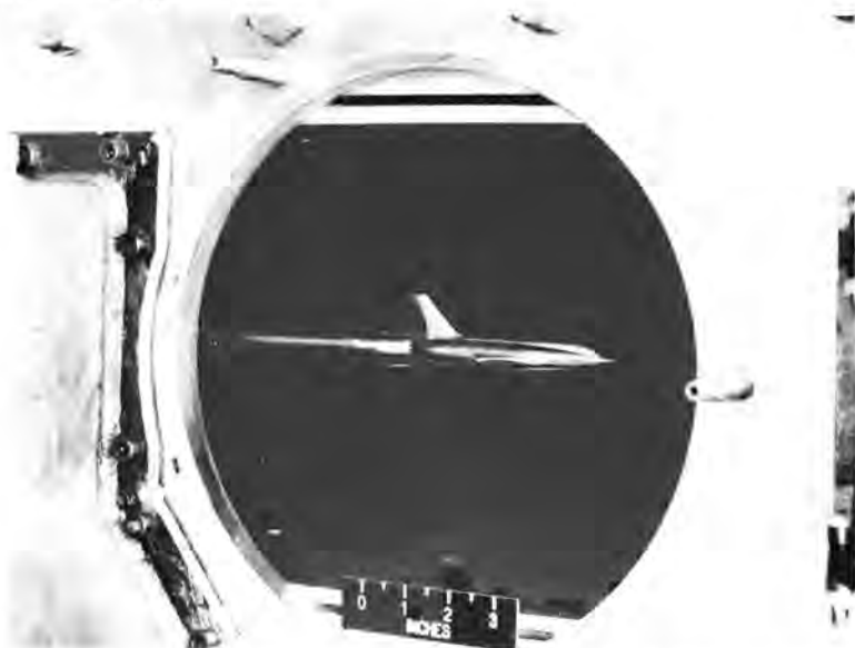
A sting-supported model of the Bell XS-2 was tested in the 9-Inch Supersonic Tunnel in July 1947.
