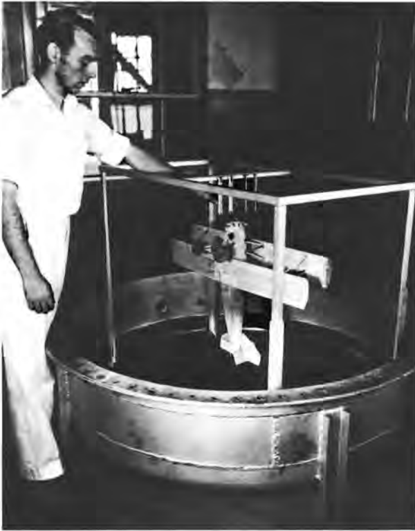
A technician mounts a model on a balance for testing in the Free-Spinning Tunnel, August 1935.
