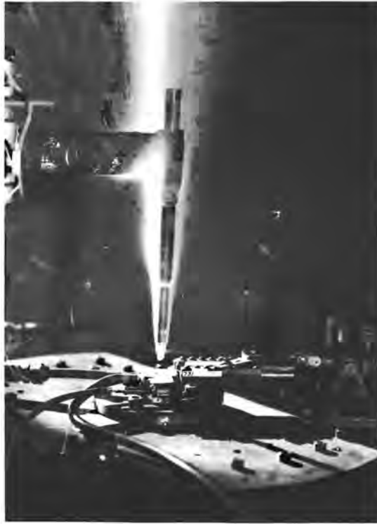
Hot-air jets employing ceramic heat exchangers played an important role at Langley in the study of materials for ballistic missile nose cones and reentry vehicles. Here a model is being tested in one of these jets at 4000 degrees Fahrenheit in 1957.
