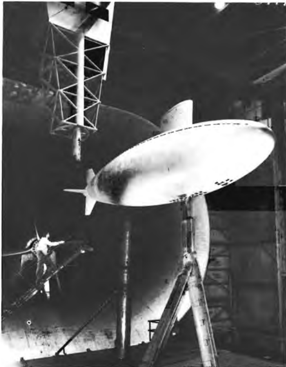
In 1950 Langley tested the drag characteristics of what was then the world's fastest submarine, the Albacore, in the FST.
