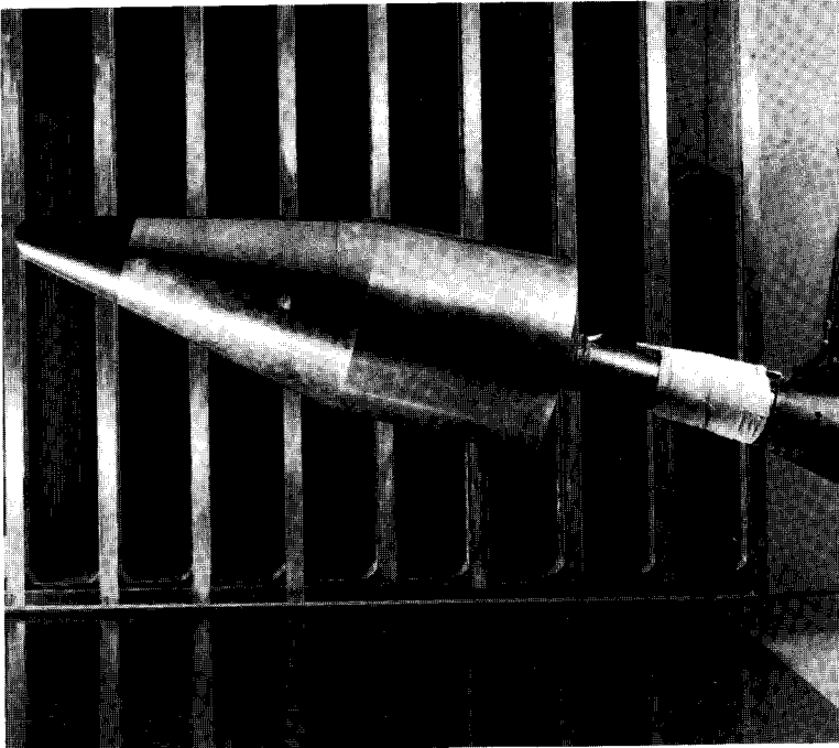
In 1957 the reentry flight path of this nose cone model of a Jupiter intermediate range ballistic missile (IRBM) was tested in the Unitary Plan Wind Tunnel.
