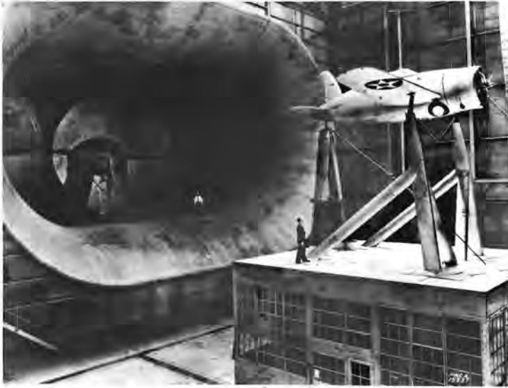
In 1938 Langley mounted the navy's Brewster XF2A-1 Buffalo in the Full-Scale Tunnel for drag reduction studies.
