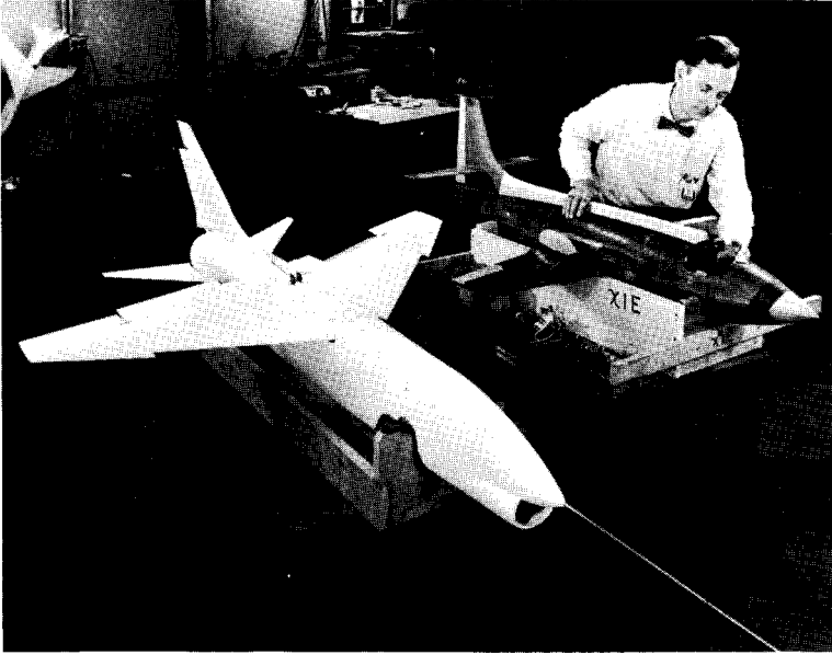
A technician prepares dynamic models of the Bell X-1E and the Vought XF-8U Crusader for wind tunnel testing in 1957. The Crusader was then the navy's fastest aircraft—maximum speed Mach 1.75 at 35,000 feet.
