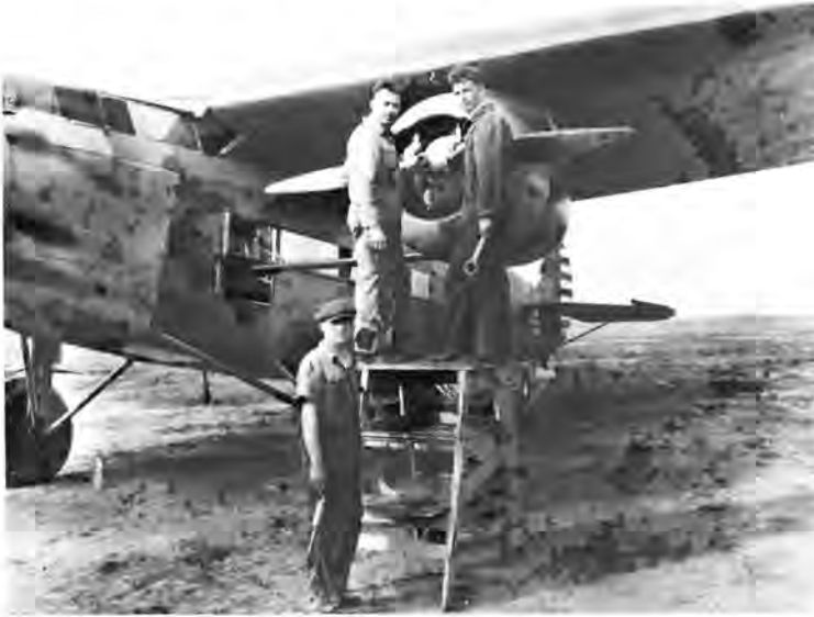
The LMAL flight crew installs an experimental low-drag cowling on the Fokker trimotor, 1929.
