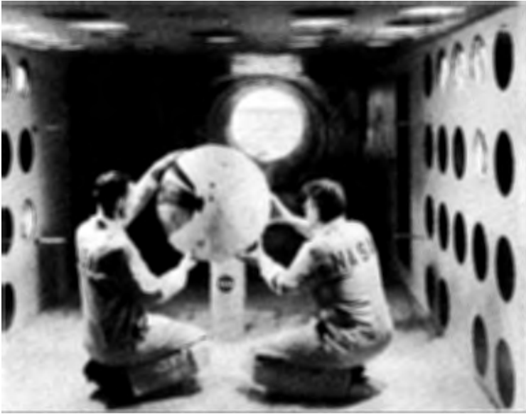
In the early 1960s the 9 × 6-Foot Thermal Structures Tunnel (top, in 1956) tested the effects of reentry heating on various space capsule materials as part of Project Fire.
