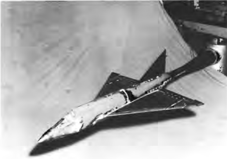
An area-rule-based model of the Convair F-102 being readied for testing in the shop of the 8-Foot HST, November 1953.
