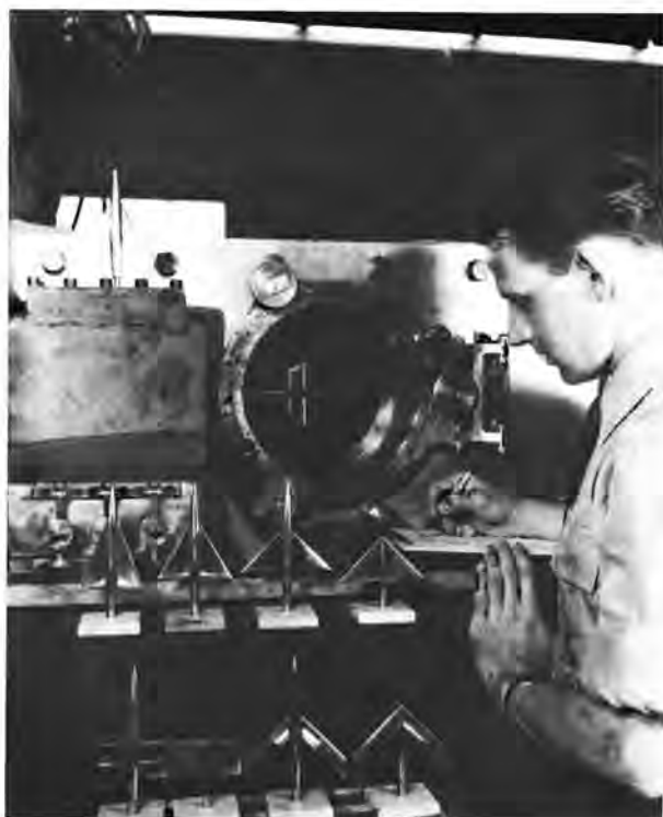
Engineer James N. Mueller tests models of various swept and delta wings in the 9-Inch Supersonic Tunnel, October 1946.
