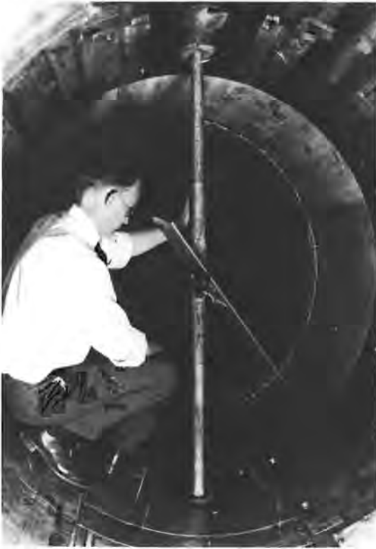
Elton W. Miller inspects damage to a wing setup in the Variable-Density Tunnel, August 1924.
