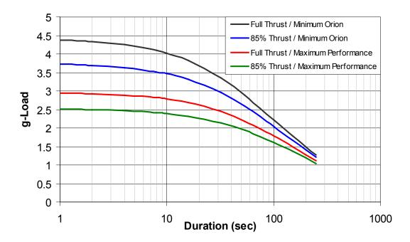
Figure 6. Orion ascent g-loading for configuration 3.
