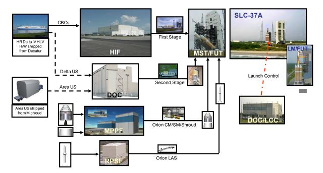
Figure 8. Option A: HR Delta IV H/Orion launch from a new SLC-37A complex.
