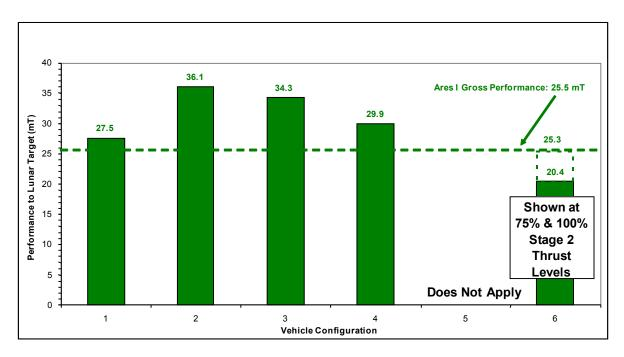
Figure 5. HR Delta IV H lift performance to lunar requirement.
