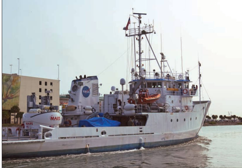
NASA utilized a number of its assets used during the Space Shuttle Program to help in performance assessment of the SpaceX C2+ mission in May 2012. The two Solid Rocket Booster Retrieval Ships, Freedom Star and Liberty Star, both carried an X-band diagnostic radar system that detects and quantifies in-flight launch vehicle behavior and any generated debris. Also on board the Freedom Star was the MARS high-powered, sea-stabilized tracking camera system that monitored the separation of the Dragon spacecraft from the Falcon 9 launch vehicle. These ships and diagnostic radar systems also helped to observe the Falcon 9 maiden flight in June 2010 and the SpaceX C1 mission in December 2010.
