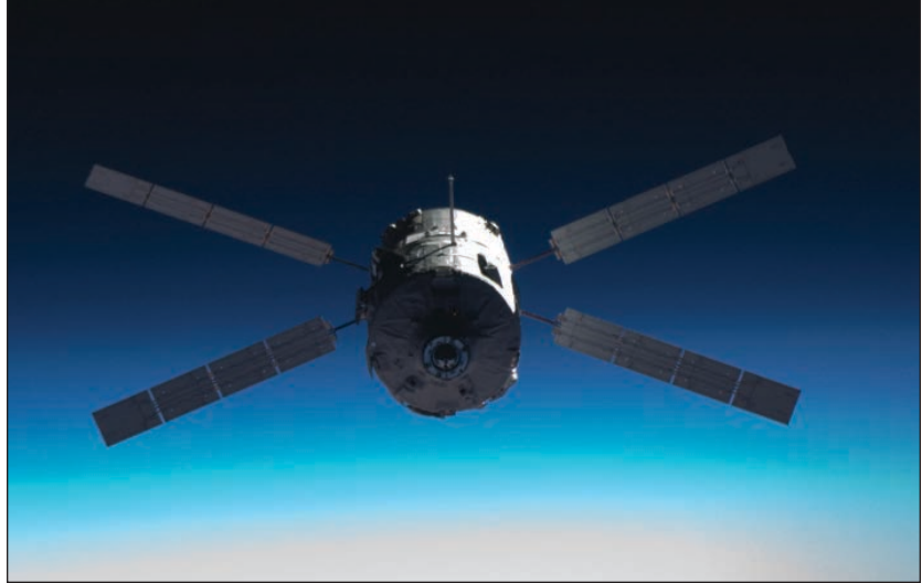
International partners provided supplies to the ISS after America’s Space Shuttle Program ended in July 2011. The European Space Agency built five Automated Transfer Vehicles (ATV), pressurized modules with a cargo capacity of almost 17,000 pounds. Shown above is the Jules Verne, the first ATV that launched March 9, 2008, and docked with the ISS on April 3. On September 29, 2008, as it reentered the Earth’s atmosphere, the ATV incinerated as planned.
