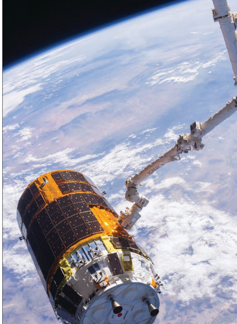
Vehicles visiting the International Space Station follow strict requirements for rendezvous, proximity operations, and berthing or docking. Adhering to these requirements was the Japan Aerospace Exploration Agency for its HTV, (pictured above), a large unmanned capacity cargo vehicle that first transferred supplies to the ISS in 2009. The vehicle's nickname, Kounotori, is the Japanese word for "white stork," symbolic of the important cargo it ferries to the astronauts living in low-Earth orbit.
