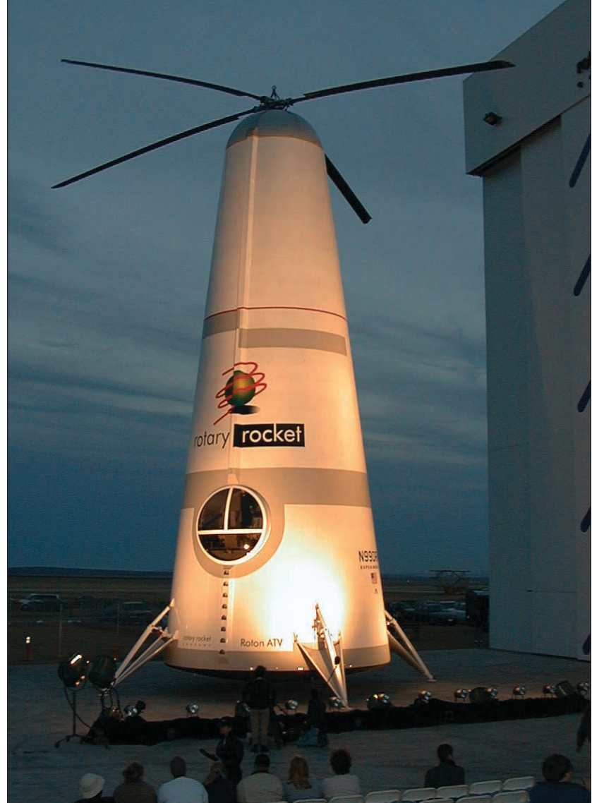
In the late 1990s, reusable launch vehicles were being commercially developed, including the Roton by the Rotary Rocket Company, Inc. The cone-shaped single-stage-to-orbit manned spacecraft featured helicopter rotor blades and an internal cargo bay.
