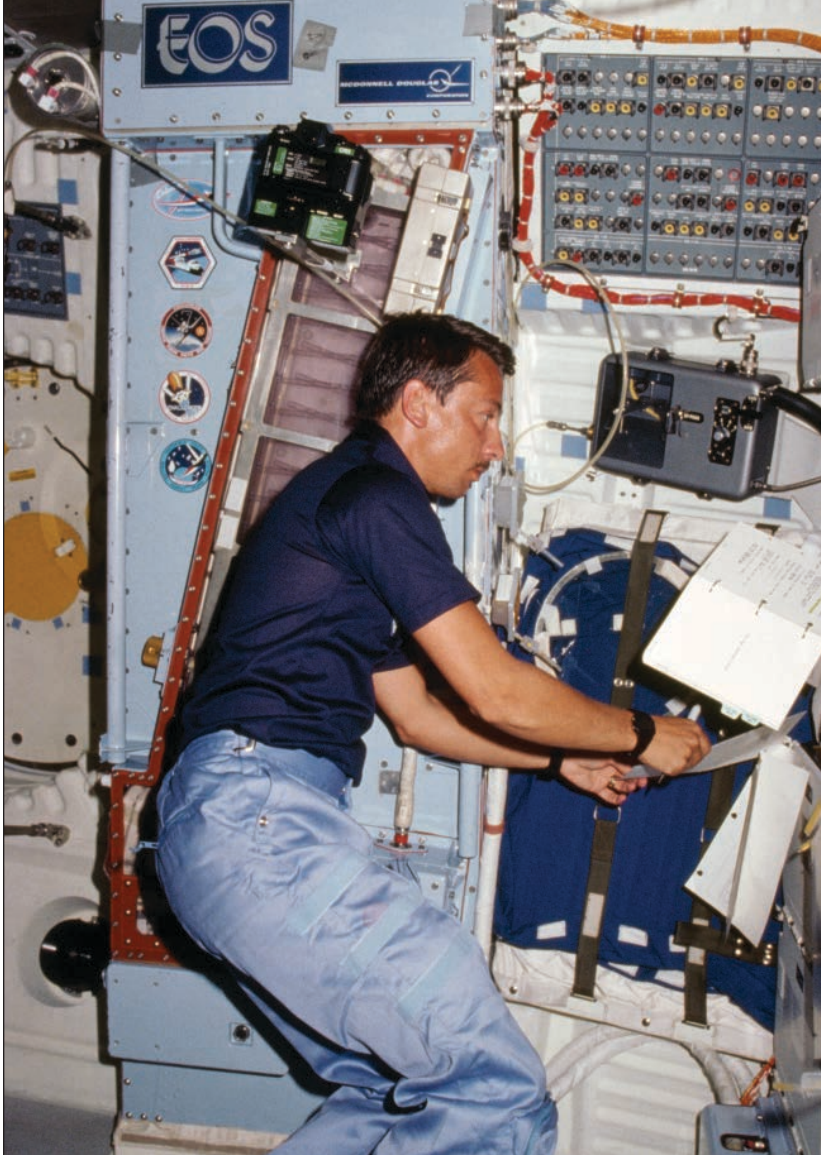
McDonnell Douglas Astronautics Company provided the first commercial experiment for the Shuttle Program – a space continuous flow electrophoresis system (CFES). The company modified laboratory instruments to take advantage of microgravity, and its engineer, Charlie Walker, operated the CFES during spaceflight. Walker (above, STS-41D) served as a payload specialist on three missions before the Space Shuttle Challenger accident that ended commercial Shuttle payloads.
