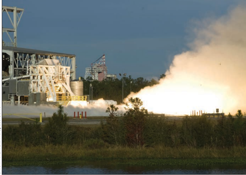
NASA Stennis Space Center in Mississippi conducted test firings on the liquid-fueled Aerojet AJ-26 engines used to power the first stage of the Orbital Sciences Corp. launch vehicle. The first in a series of three firings, this test (pictured above) on November 11, 2010, was held to verify start and shutdown sequences on the engines, along with test stand operations and ground-test engine controls.
