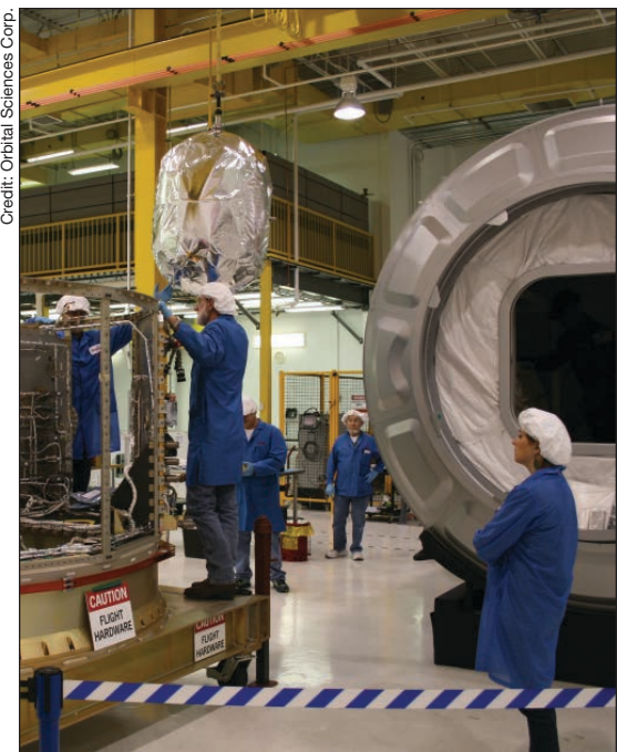
By using an overhead crane, Orbital’s integration and test engineers lifted one of the three main propellant tanks into the structure of the Cygnus Service Module. This Service Module was flown on the COTS Demonstration Mission that was successfully completed in October 2013.
