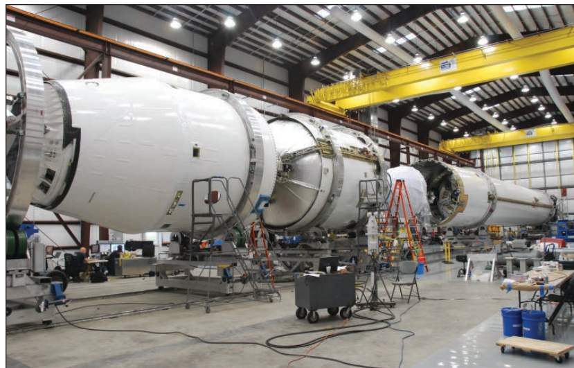
Prior to its inaugural launch, the Falcon 9 rocket undergoes its final integration in the hangar at SpaceX's Cape Canaveral launch site in Florida. Components include: Dragon spacecraft qualification unit (left), second stage with Merlin vacuum engine (center), first stage with nine Merlin 1C engines (right).
